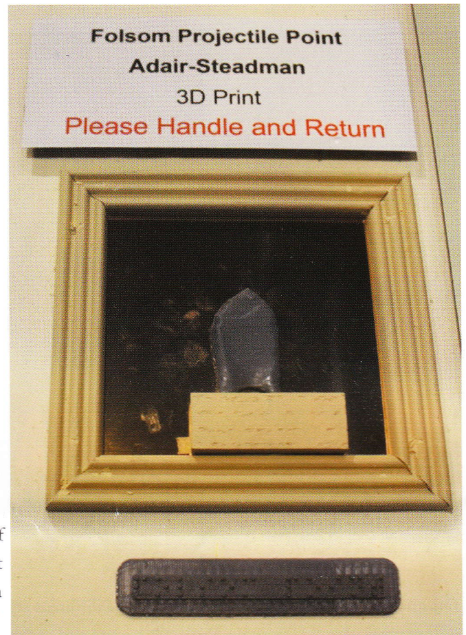
Figure 2. A capacitive touch sensor plays a recorded audio message of the 3D modeled projectile point.
